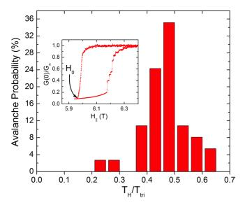
FIG. 3. (Color online) A histogram of the avalanche probability as a function of the normalized nonequilibrium Zeeman temperature (see text). The avalanche statistics were collected from six tunneling DOS hysteresis loops that were measured consecutively with identical field sweep protocols. Inset: A typical hysteresis loop used to collect the statistics in the main figure. The arrow indicates the low-field closure point of the loop,  $H_0$ .
