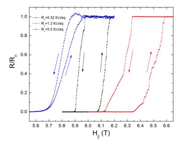
FIG. 1. (Color online) Parallel critical field transitions measured at 60 mK for three Al films of varying normal-state sheet resistance. The sheet resistance of each film has been normalized by its normal state value.
