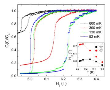
FIG. 4. (Color online) Hysteresis in the normalized zero-bias tunneling conductance of the film in Fig. 2 at various  $T < T_{\rm Tri}$ . Inset: The upper and lower parallel critical fields as a function of temperature determined from the midpoint of the critical field transitions as obtained from the zero-bias tunneling conductance.
